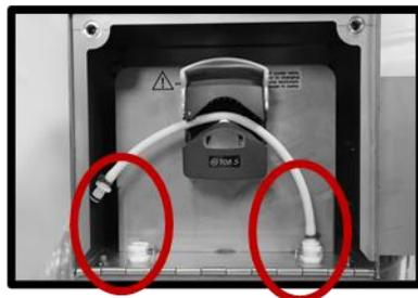
5. Press in the silver tab at the end of the pump tube and release the one side of the pump tube.
