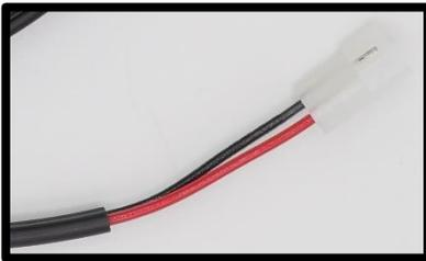
3. Part #364C has a white plug on one end. Connect this output wire connection to the SP-2L Control. On the SP-2L Control, the wire lead will be orange (+) and blue (-).
