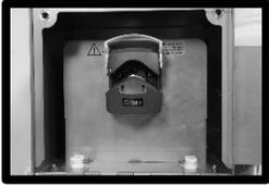
7. Remove the pump tube.
