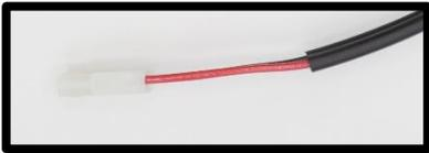
2. The other end of Part #364A has a white plug on it. This plug will mate up to the input wire connection on the SP-2L Control. On the SP-2L Control, the wire lead will be black (-) and red (+).
