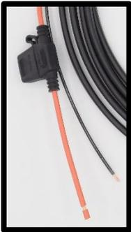
• **ORANGE WIRE (w/FUSE HOLDER):** The orange/red wire must be connected to 12 volt DC positive (+). It is recommended this be connected to a 12 volt DC regulated power source, such as an in-cab power outlet, or a header switch output. If wiring into a “header switch” output, the red wire should be connected to the 12 volt DC (+) switched output. **Only install a 3 AMP Fuse into the fuse holder.**
