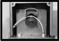
9. Push end of the tube into the hole until you hear it **CLICK** into place.
