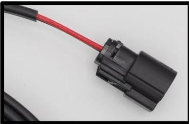
4. From here, Part #364C will be routed to the pump assembly. On the bottom of the pump assembly, you will find a black plug. The black plug on the end of Part #364C will connect here. The plug can only connect one way. Mate up the plug and insert until it **CLICKS**. Additional details on **Page 11**.
