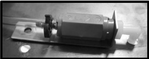
5. Now, mark the spot where the nut and bolt will be used to secure the bracket. If you need to, remove the hose before marking and drilling.
