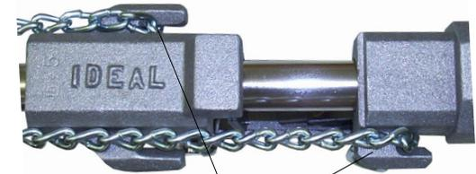
If performing a single pull, attach one chain to a hook on the bottom half of the jack and one chain to the hook on the opposite side of the jack. The single hook on the top half of the jack is not used for the single pull (see right).
